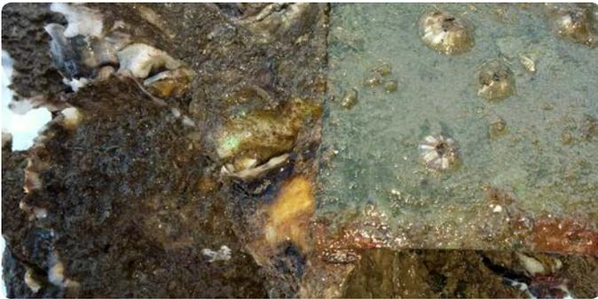
**A:** Massive attachment to uncoated side of coupon after 18 months submersion
