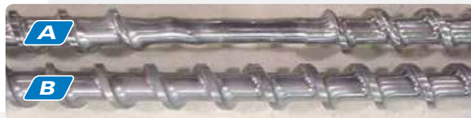
CarbideX Coated Feedscrew with Mirror Finish
