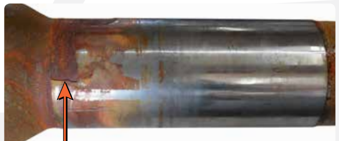
Standard coated spline mandrel. Typical Issue: failure due to chloride attack, causing cracking and chipping
