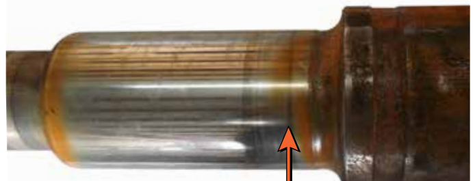
Standard bearing mandrel. Typical Issue: wearing at lower seal
